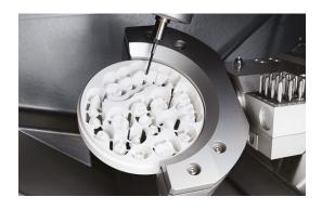
Another novelty is the integrated water cooling, which significantly minimizes the thermal expansion of the spindle and Z axis. Faster machining with even more consistent results and longer spindle lifes are the benefits for future SilaMill R5 owners.
